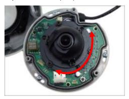
4. Tighten the three (3) screws to fix the pan position.
