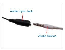
**NOTE:** The microphone must have a built-in amplifier. Connecting an ordinary microphone will dwarf sounds and will result in inaudible recording.
