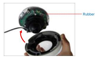
**NOTE:** Make sure the rubber on the camera is positioned properly on its track as the dome cover is closed on the camera to ensure protection against water ingress.
