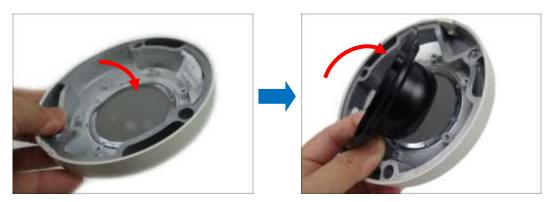
6. Align the screw holes and secure the six (6) screws.
