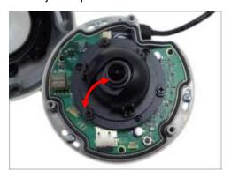
**NOTE:** Because the lens is secured tightly to the module, users need to push hard to tilt the lens.
