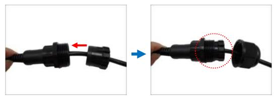
8. Attach the clamping nut to the cable gland body. Make sure the clamping nut is tightly secured and the rubber is squeezed in to avoid water leakage.
