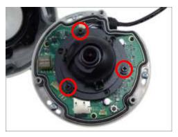
3. Turn the lens module to adjust the camera pan position.
