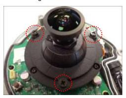
3. Turn the lens module to adjust the viewing orientation. The arrow on the lens indicates the top side orientation.
