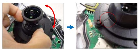
4. Once done, tighten the three (3) screws to fix the lens position.
