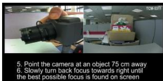
TCM-5311 back focus adjustment with PLEN-0203
